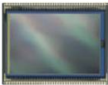
APS-H size sensor; approx. 29 x 19mm
